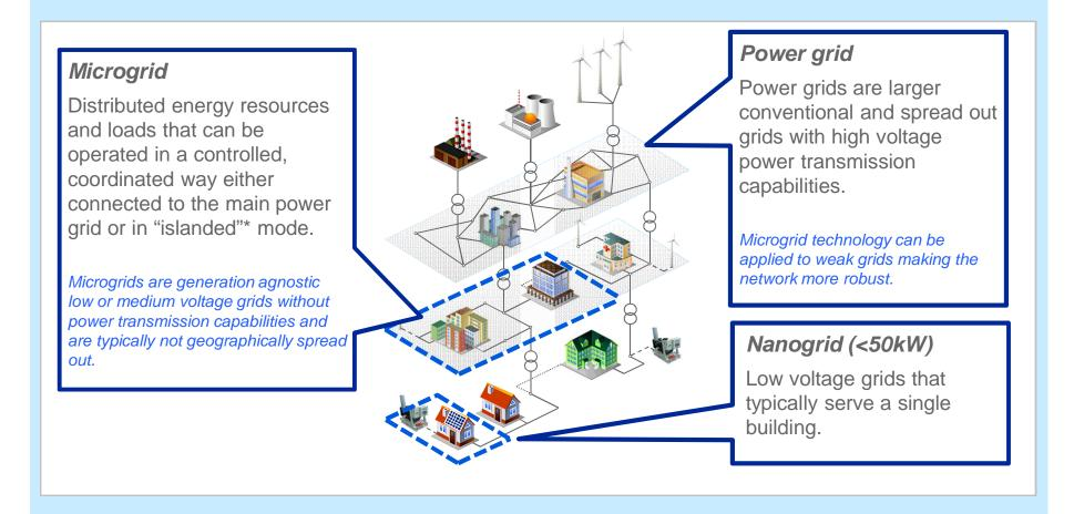
Islanded mode: ability to provide power independently from the main power grid
