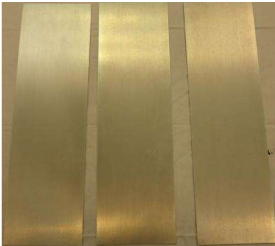
Figure 85 – Alodine T 5900 RTU, 2139 – 2142
