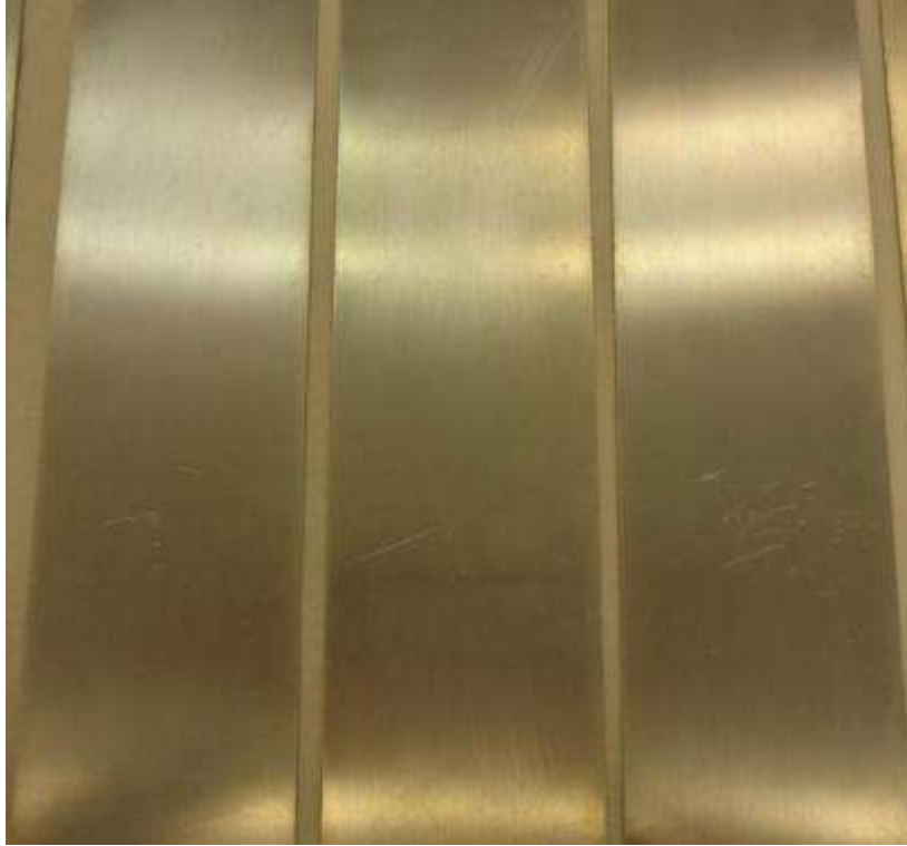
Figure 117 – Alodine T 5900 RTU, 2024-T3
