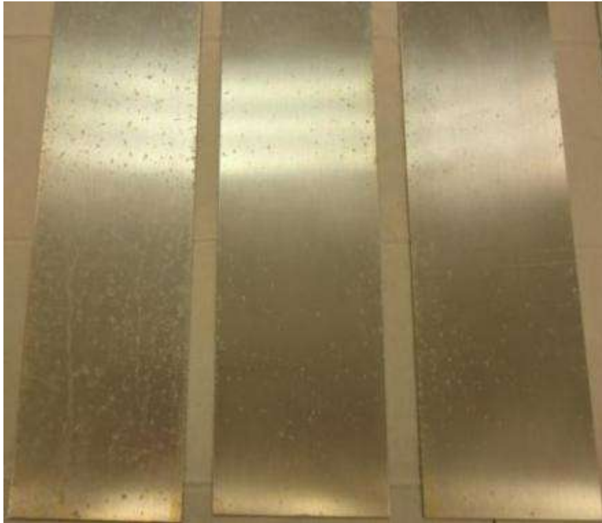
Figure 84 – Alodine T 5900 RTU, 2100 – 2102
