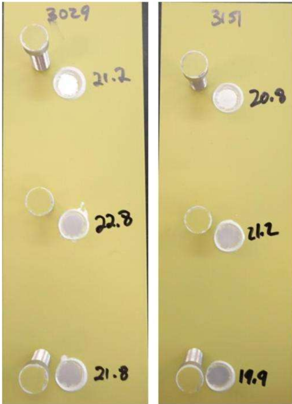
Figure 142 – Iridite NCP; 6061-T6 (Left), 5052-H32 (Right)
