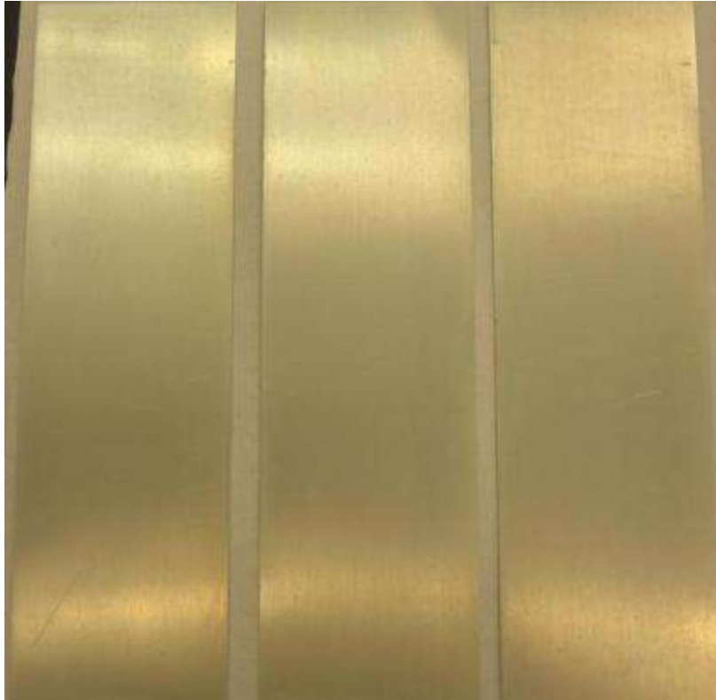
Figure 115 – Alodine T 5900 RTU, 6061-T6
