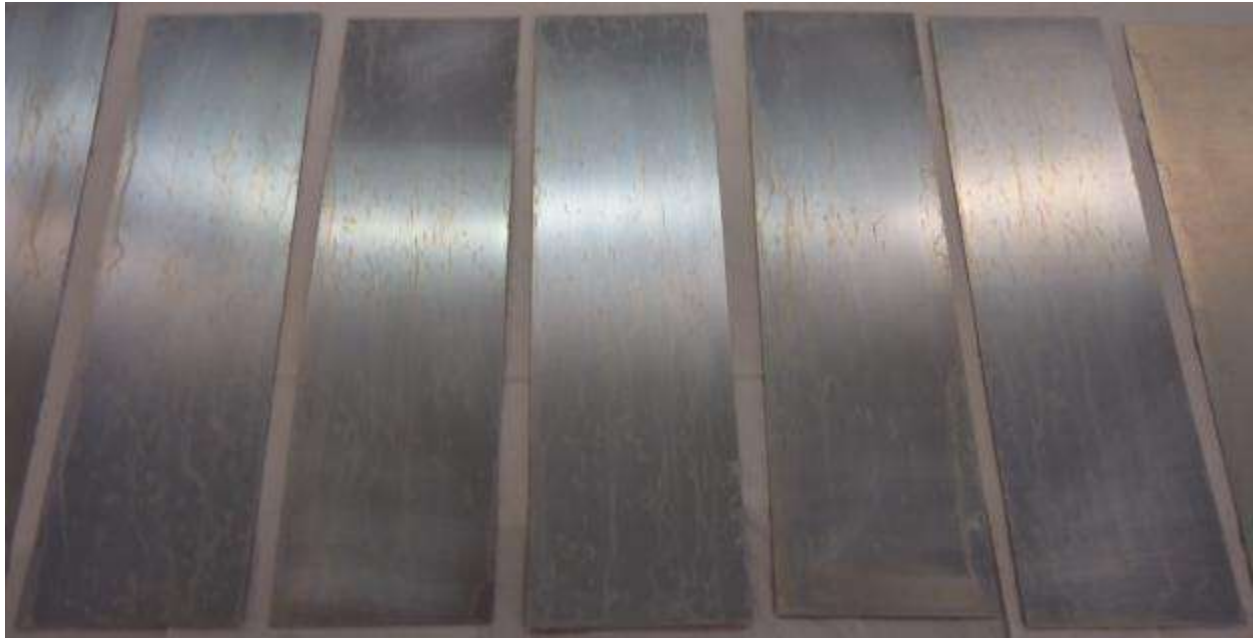
Figure 14 - Alodine T 5900 RTU, 2089 – 2093
