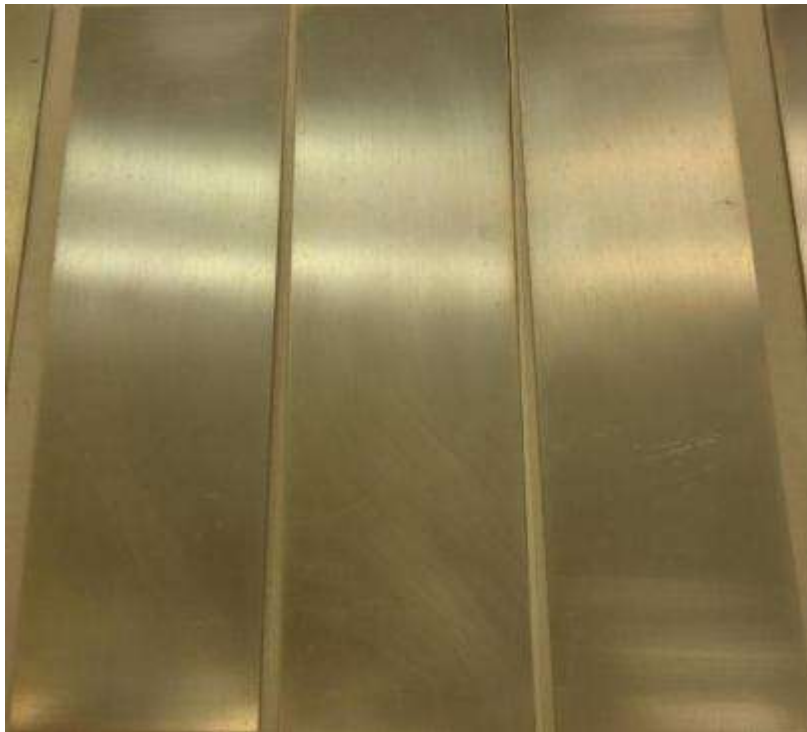
Figure 116 – Alodine T 5900 RTU, 7075-T73
