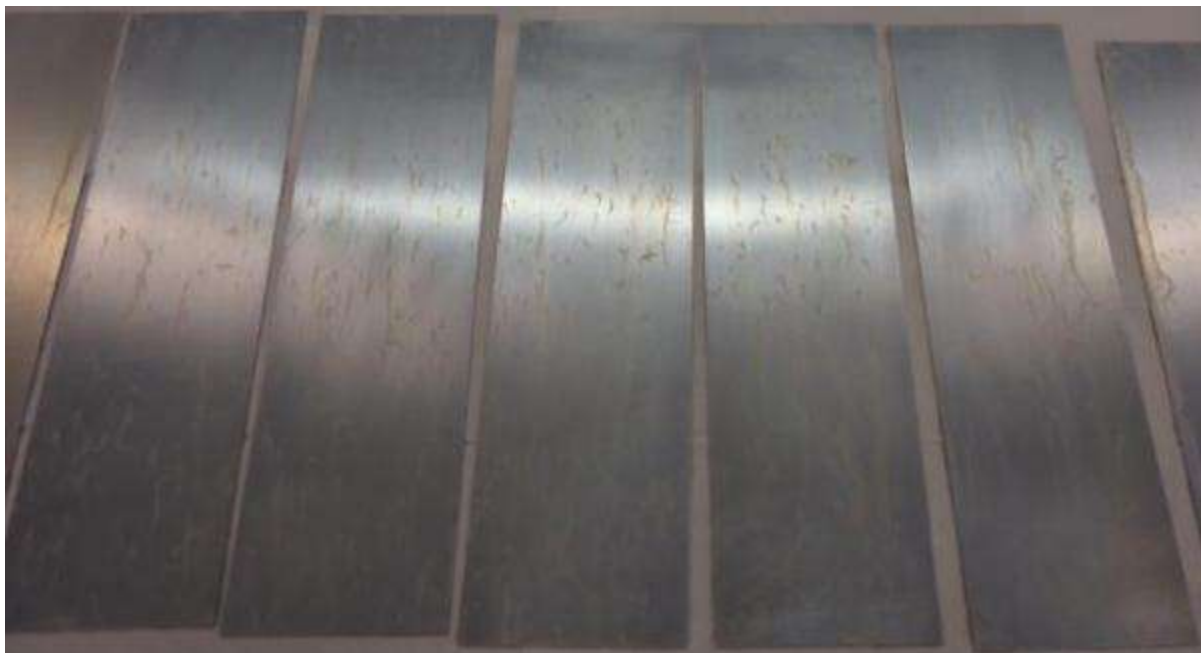
Figure 13 - Alodine T 5900 RTU, 2051 – 2055
