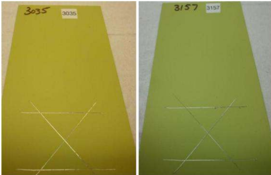
Figure 172 – Iridite NCP - ; 6061-T6 (Left), 5052-H32 (Right)
