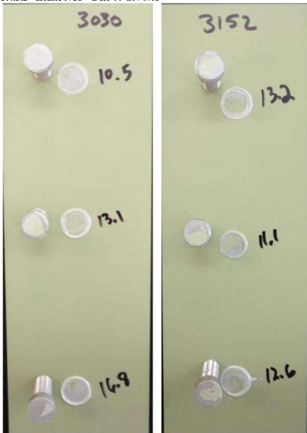
Figure 148 – Iridite NCP; 6061-T6 (Left), 5052-H32 (Right)
