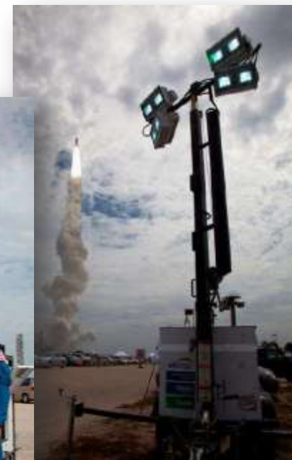
Fuel cell mobile light in support of final Shuttle launch (Atlantis), July 2011
