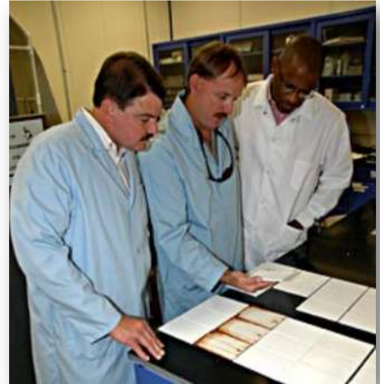
Inside the Corrosion Technology Lab at NASA KSC, workers from TEERM are comparing several coating test samples with some new environmentally friendly coatings.
