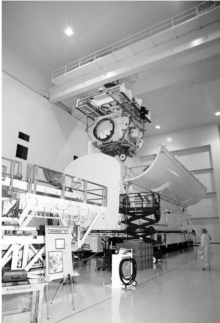
Figure A-16. The Z1 Truss being loaded into a payload canister to be transported to the launch pad where it will be installed in the orbiter, camera facing southwest, September 11, 2000.
