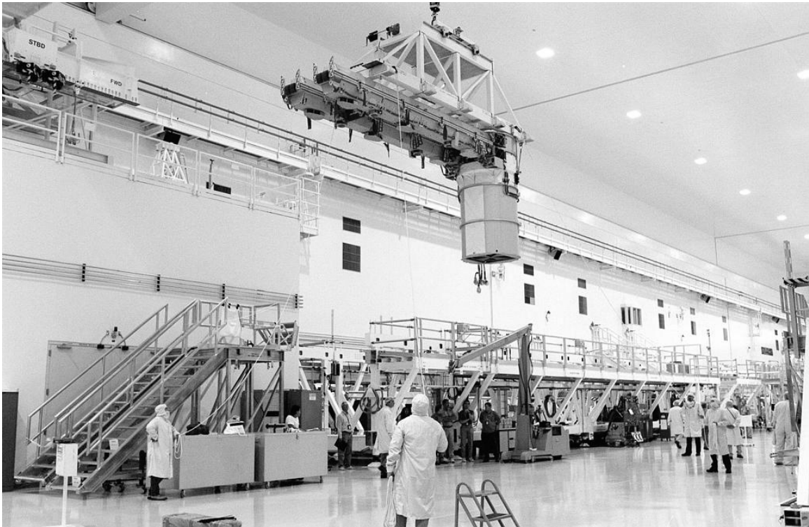
Figure A-21. Solar panels for the ISS being carried to their designated workstand in the SSPF High Bay, camera facing northeast, December 7, 1998. Source: NIX, http://nix.nasa.gov/ , KSC-98PC-1855.
