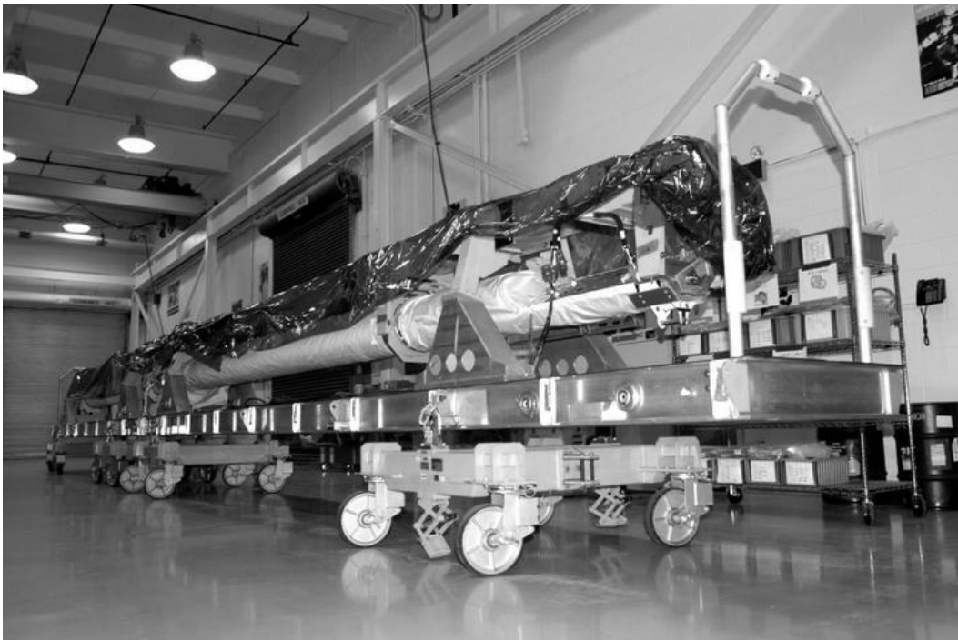
Photo A-19. The Orbiter Boom Sensor System in the RMS lab for testing, 1 January 2005. Source: John F. Kennedy Space Center, KSC-05PD-0063, accessed via http://mediaarchive.ksc.nasa.gov/search.cfm .
