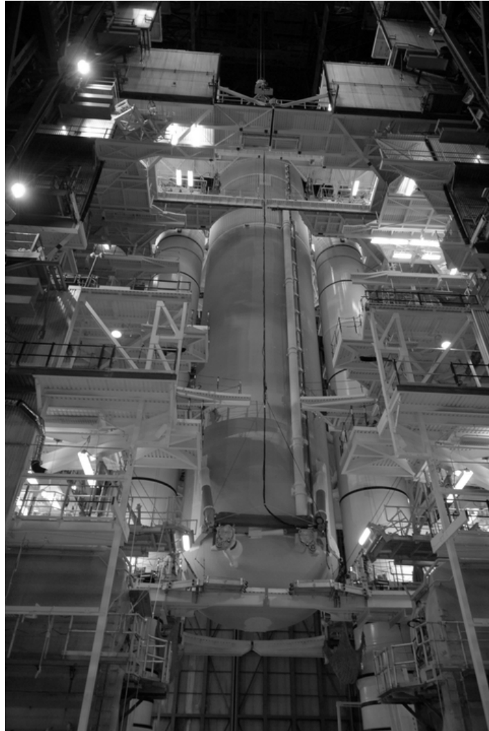
Photo A-12. External Tank being lowered to mate with SRBs, 28 August 2008. Source: John F. Kennedy Space Center Archives, KSC-08PD-2525, accessed via http://mediaarchive.ksc.nasa.gov/search.cfm .
