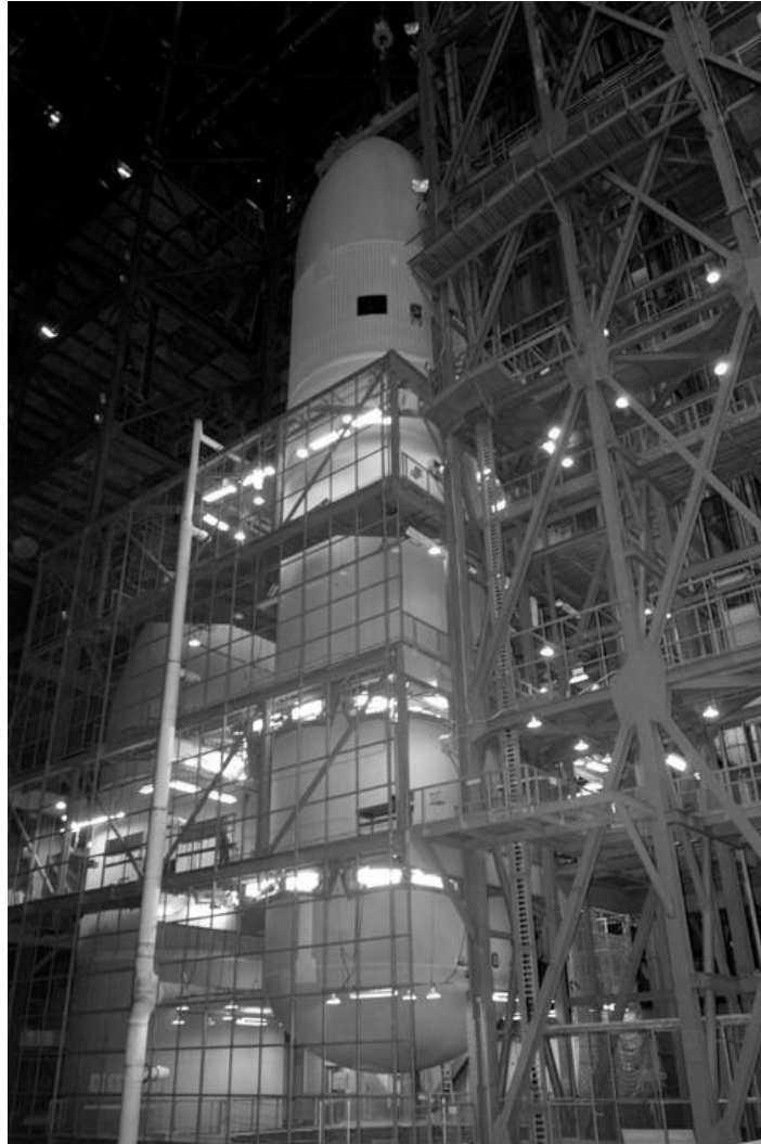
Photo A-11. External Tank being removed from check-out cell for mating to SRBs, 28 February 2005.
