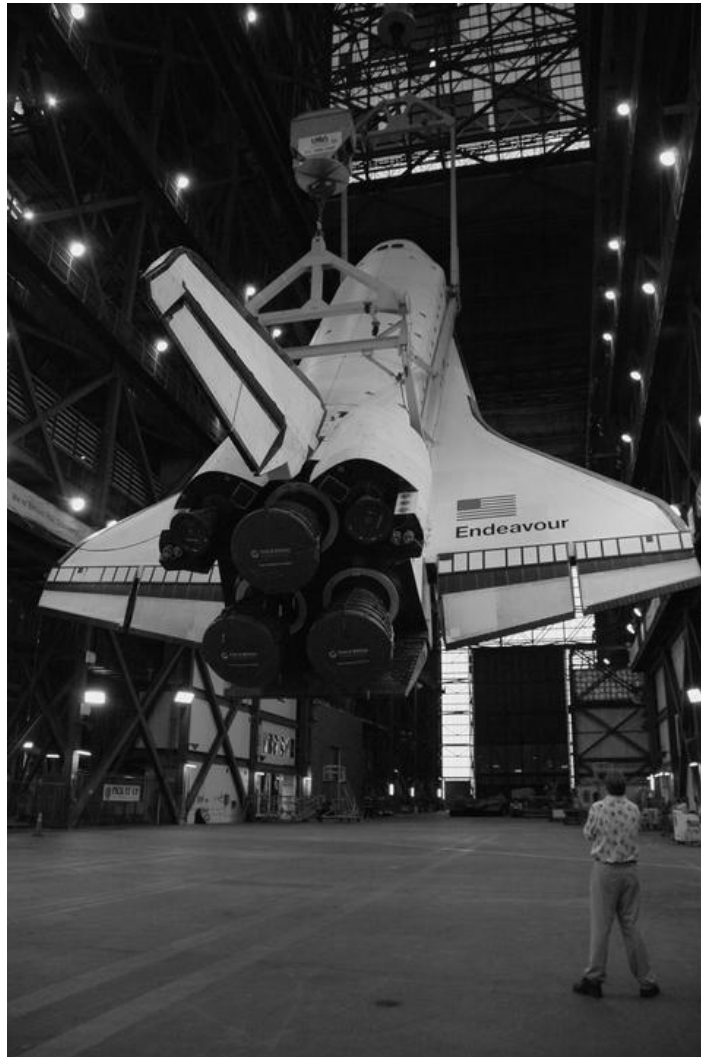
Photo A-14. Orbiter Endeavour being rotated to vertical in transfer aisle, 7 July 2007. Source: John F. Kennedy Space Center, KSC-07PD-1754, accessed via http://mediaarchive.ksc.nasa.gov/search.cfm .
