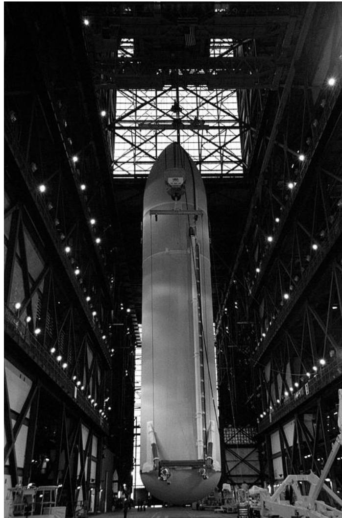
Photo A-8. External Tank after it has been rotated to vertical and is ready to be moved into one of the ET check-out cells, 9 February 1999.
