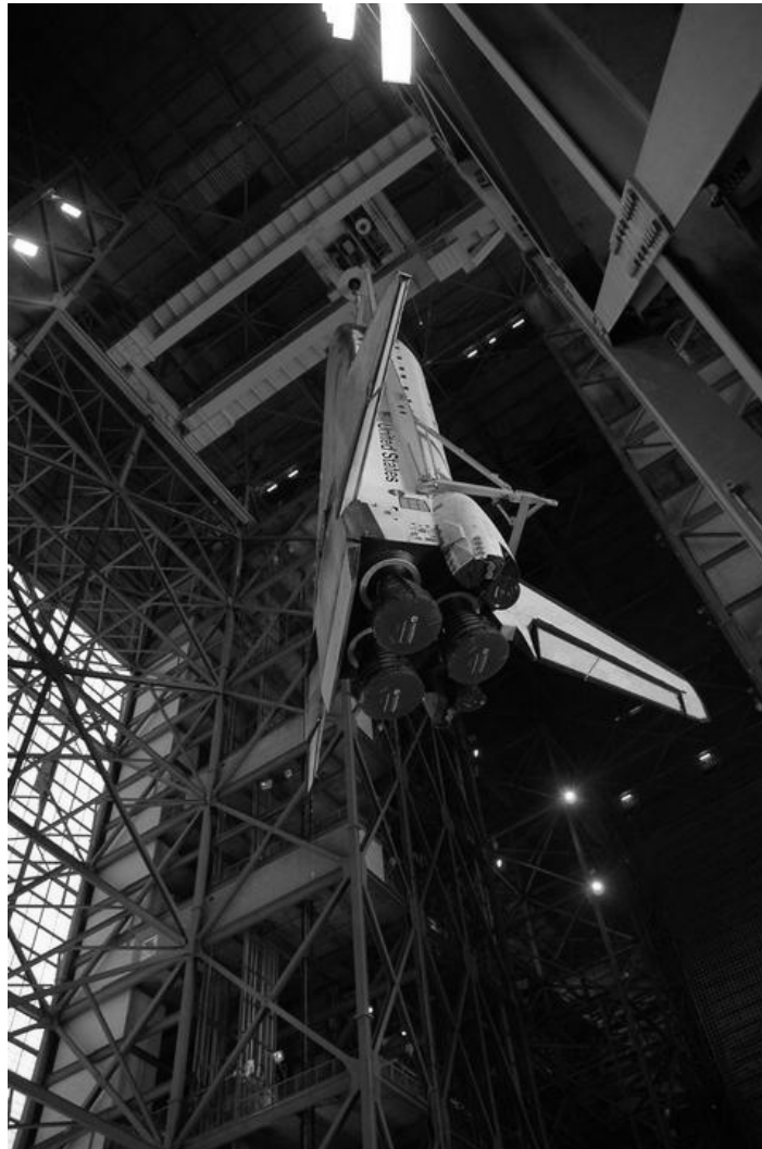
Photo A-15. Orbiter Endeavour being moved from transfer aisle to high bay, note the 45 degree angle of the orbiter to fit through the diaphragm, 7 July 2007.
