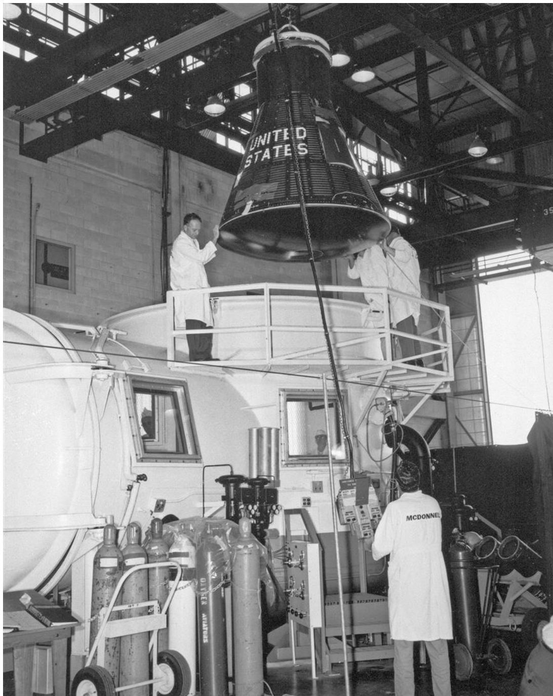
Figure 7. Mercury Capsule #16 being moved into the altitude chamber in Hangar S, 1962. (Courtesy of Kennedy Space Center Archives, Image LOC-62-3051).
