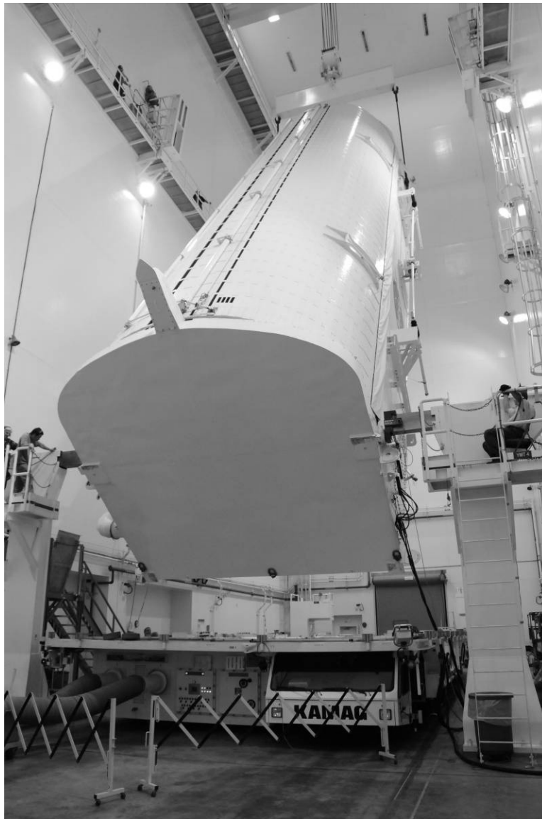
Figure A-16. View showing the rotation process of the payload canister approximately two-thirds complete, April 13, 2010. Source: Penny Rogo Bailes.
