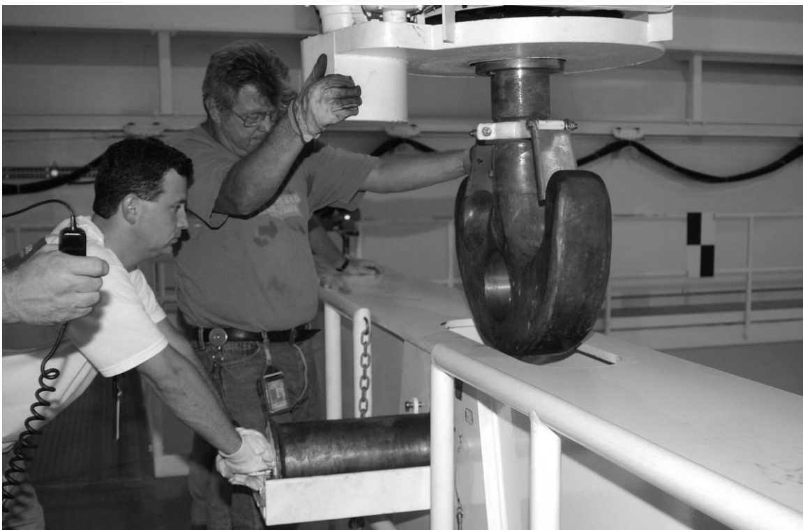
Figure A-11. Detail view showing crane hook being lowered into the slot on the lifting beam; the technician at the left is maneuvering the locking pin. Source: "Inside the Canister Rotation Facility." Spaceport News (41, 1), January 11, 2002: 4.
