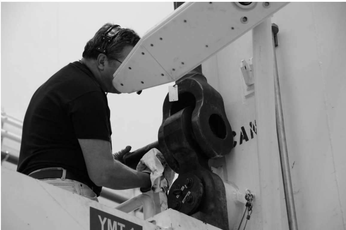
Figure A-13. Detail view showing a sling being fitted around a forward lug retainer, April 13, 2010.
