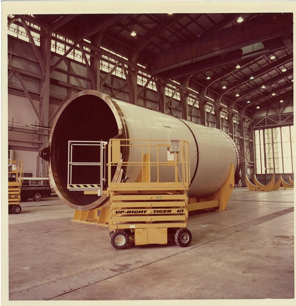
Figure 15. SRB Solid Rocket Motor (SRM) segment inside Hangar AF, 1979. (Courtesy: KSC, Image 108-KSC-379C-1061/9).
