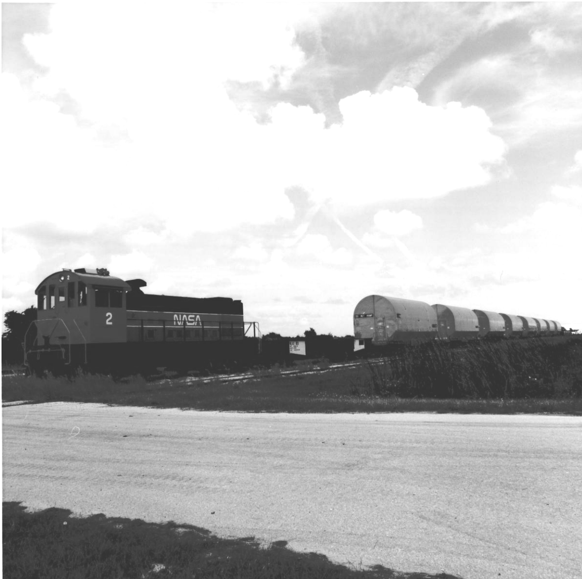
Figure A-10. Alco locomotive hauling SRM segments, October 21, 1982. Source: John F. Kennedy Space Center Transportation Office, 108-KSC-382C-3683.4.
