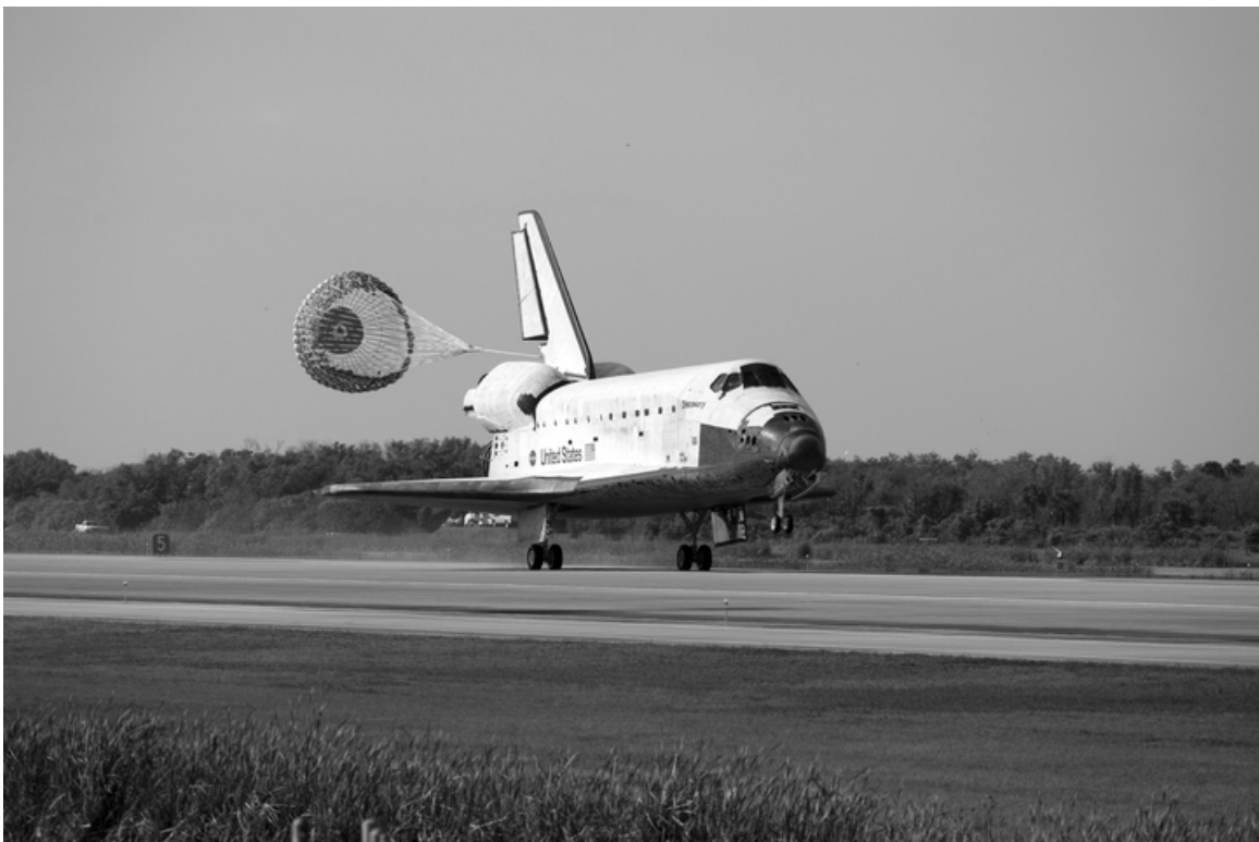
Figure A-20. The Orbiter Discovery , with drag chute deployed, bringing nose landing gear down onto the SLF Runway, camera facing southwest, April 20, 2010.
