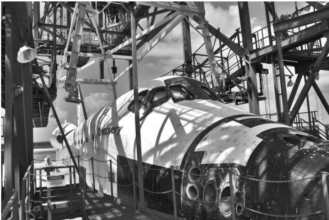
Figure A-24. The MDD slingback is prepared to be lowered around Discovery , camera facing northwest, August 21, 2005.
