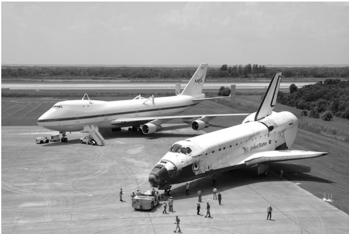
Figure A-26. Discovery being pushed onto the SLF parking apron by a tug following demating operations (the SCA is in the background), camera facing west, August 22, 2005.
