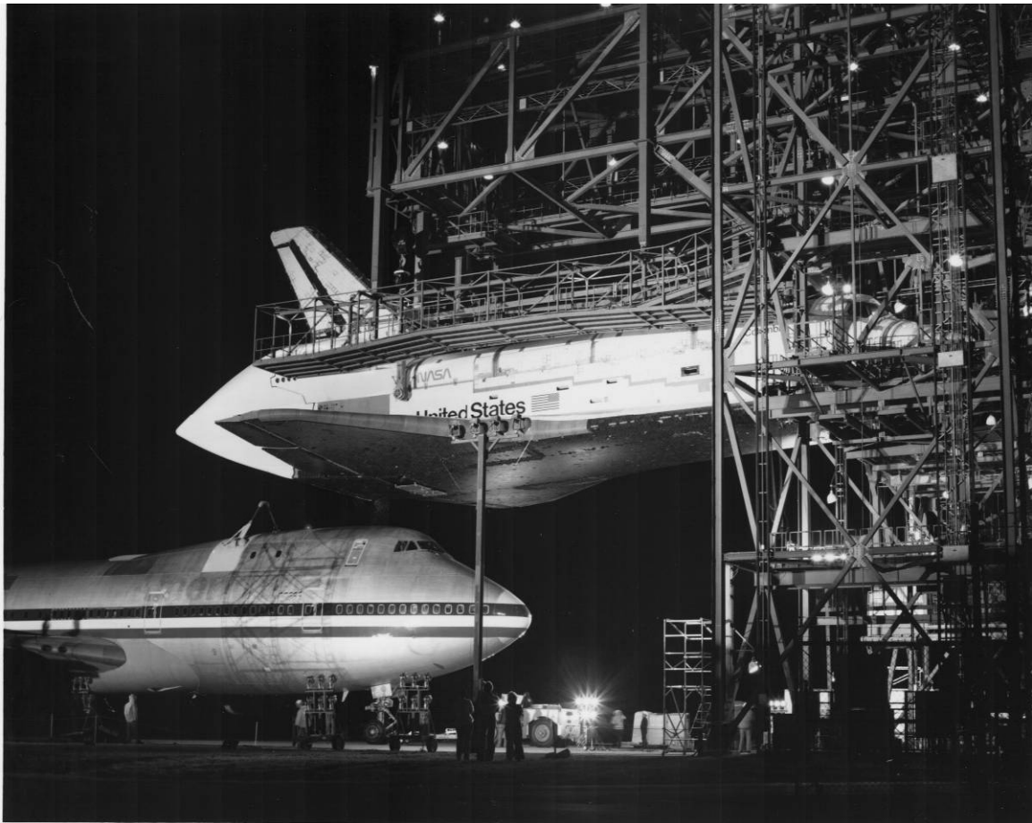
Figure A-14. The SCA being cleared from the MDD area as Columbia is held in place by the slingback, camera facing northwest, March 25, 1979. Source: John F. Kennedy Space Center Archives, 108-KSC-79PC-60.
