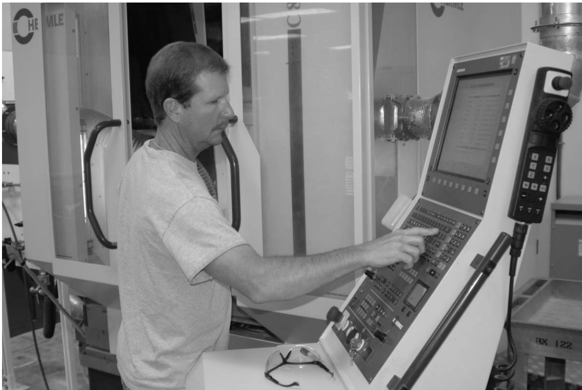
Figure A-7. A KSC tile technician loading specifications into the fully-automatic Milling Machine, March 9, 2010. Source: Penny Rogo Bailes.
