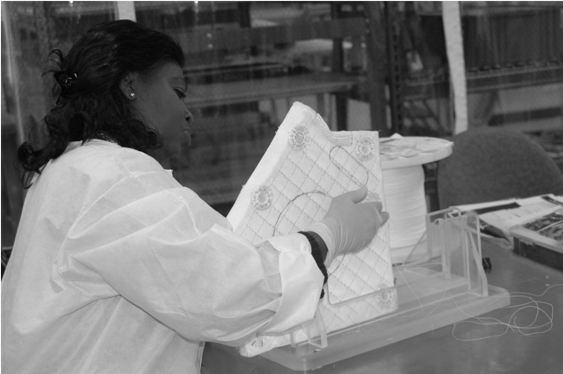
Figure A-30. Custom FRSI blanket being hand-sewn by a KSC technician, March 9, 2010. Source: Penny Rogo Bailes.
