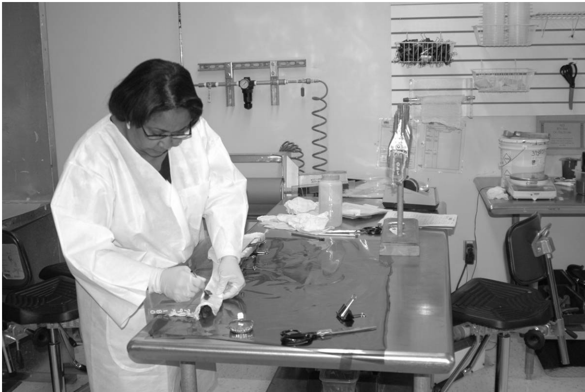
Figure A-22. RTV being applied to softgoods material by a KSC technician, March 9, 2010. Source: Penny Rogo Bailes.
