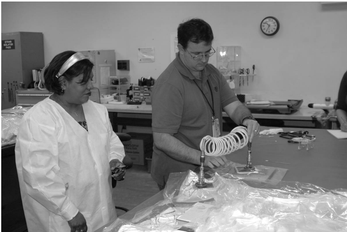
Figure A-20. Bag with SIP/tile being fitted with vacuum lines by technician Kay Sunderman and a KSC quality control manager, March 10, 2010. Source: Penny Rogo Bailes.
