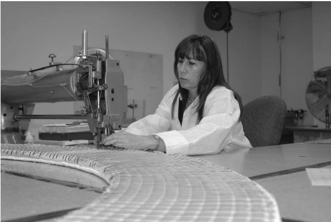
Figure A-28. Arced FIB being sewn on Long-Arm Sewing Machine by technician Kathy Evans, March 9, 2010. Source: Penny Rogo Bailes.
