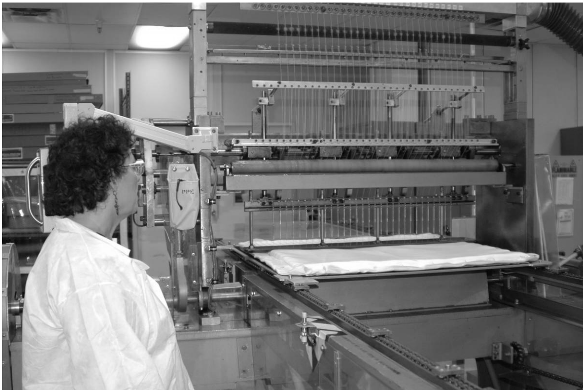
Figure A-25. FIB being sewn by Multi-Needle Sewing Machine under the watchful eye of technician Jean Wright, March 9, 2010.
