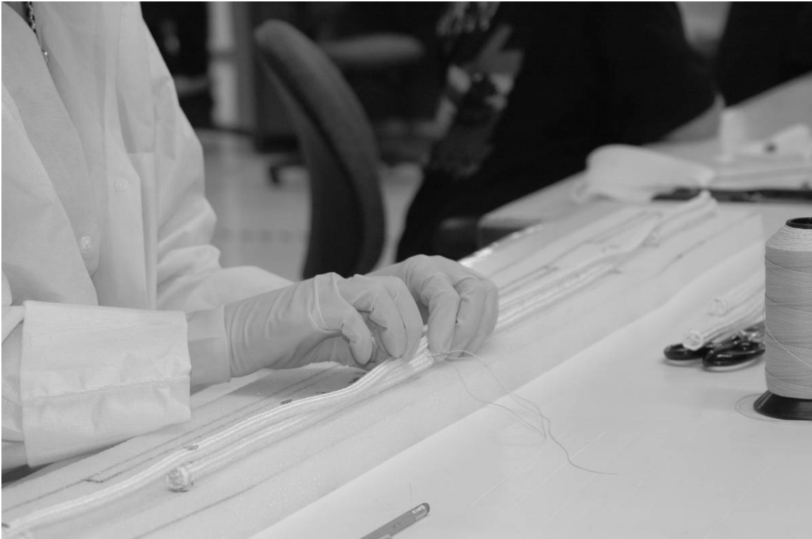
Figure A-32. Detail of thermal barrier being hand-sewn by a KSC technician, March 9, 2010. Source: Penny Rogo Bailes.
