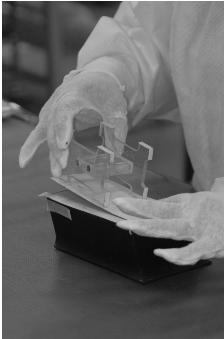
Figure A-18. SIP being positioned on a tile by technician Kay Sunderman, March 10, 2010. Source: Penny Rogo Bailes.
