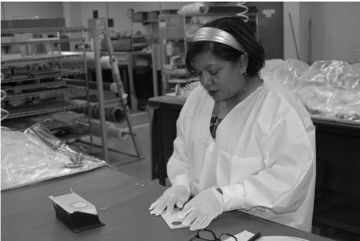
Figure A-16. SIP being prepared for bonding to a tile by technician Kay Sunderman, March 10, 2010.
