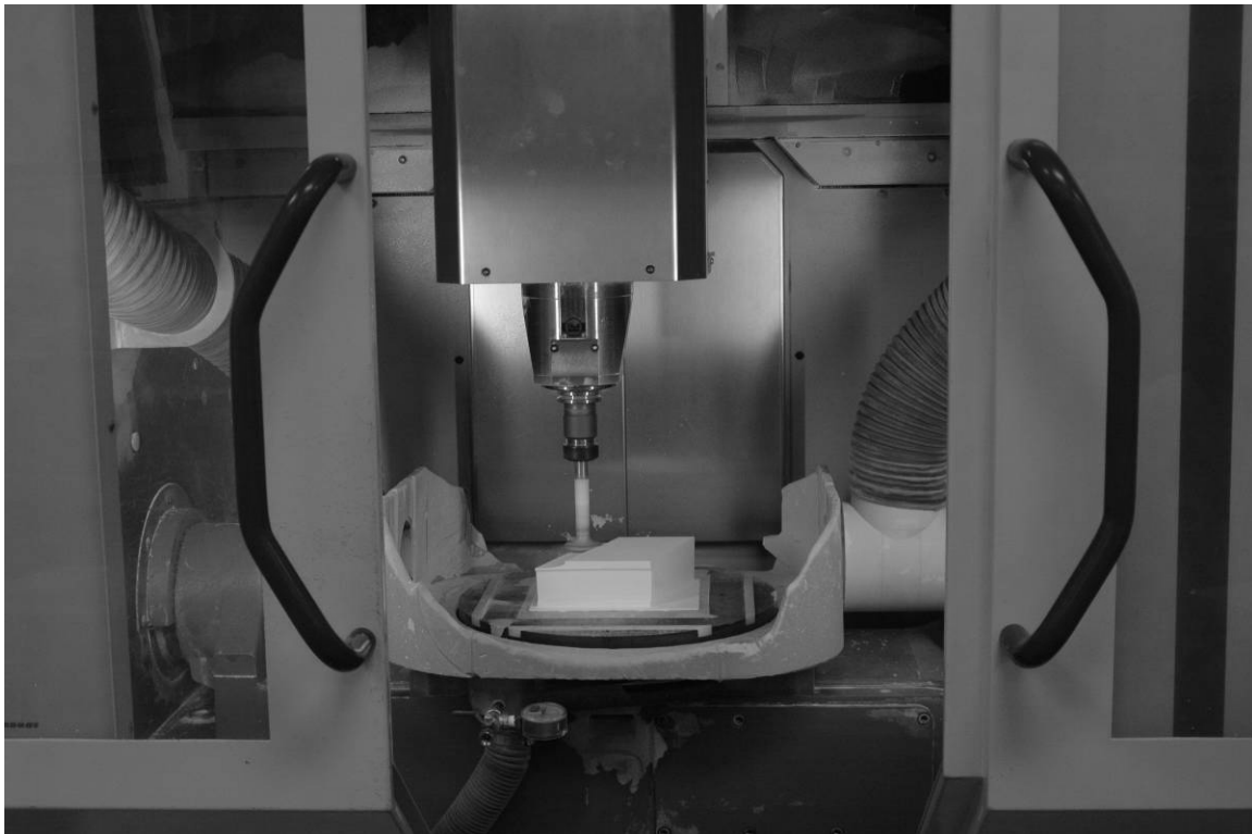
Figure A-9. Tile being cut by the fully-automatic Milling Machine, March 9, 2010. Source: Penny Rogo Bailes.
