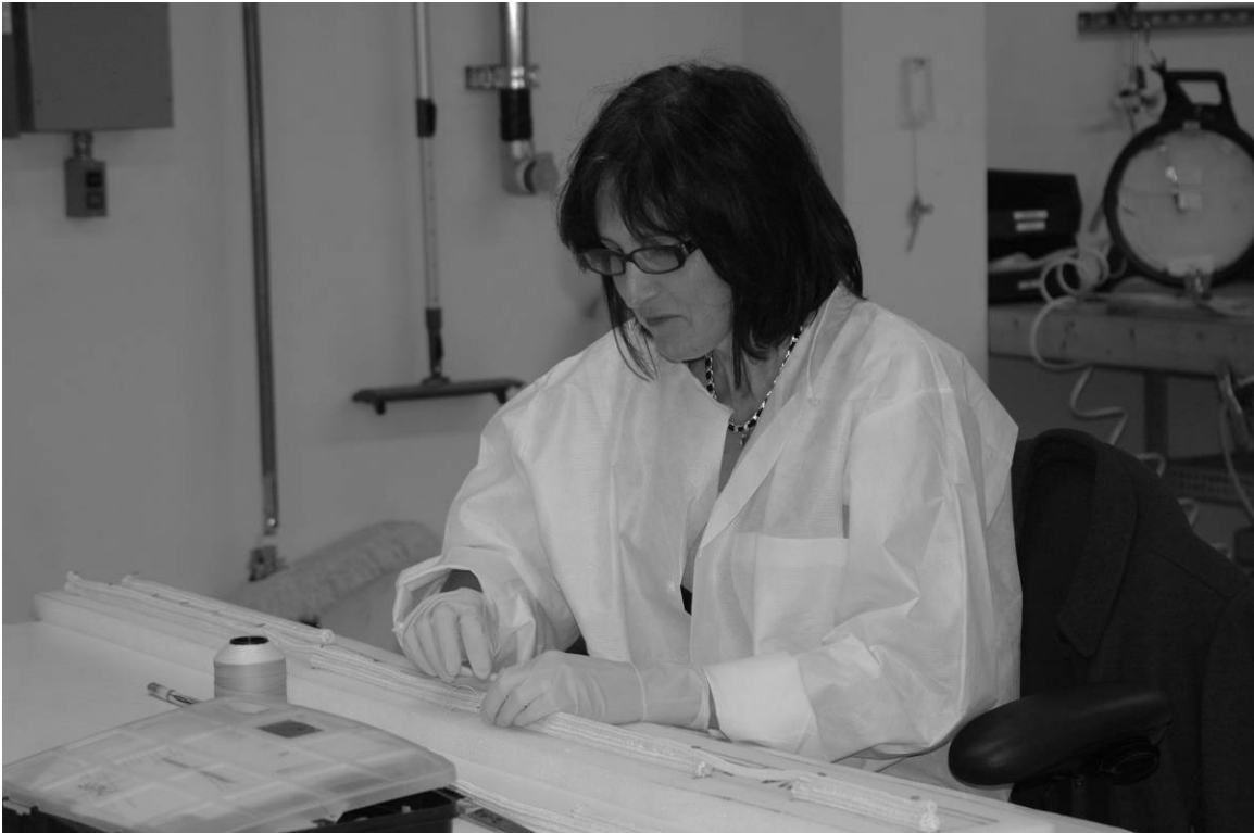
Figure A-31. Thermal barrier being hand-sewn by a KSC technician, March 9, 2010. Source: Penny Rogo Bailes.
