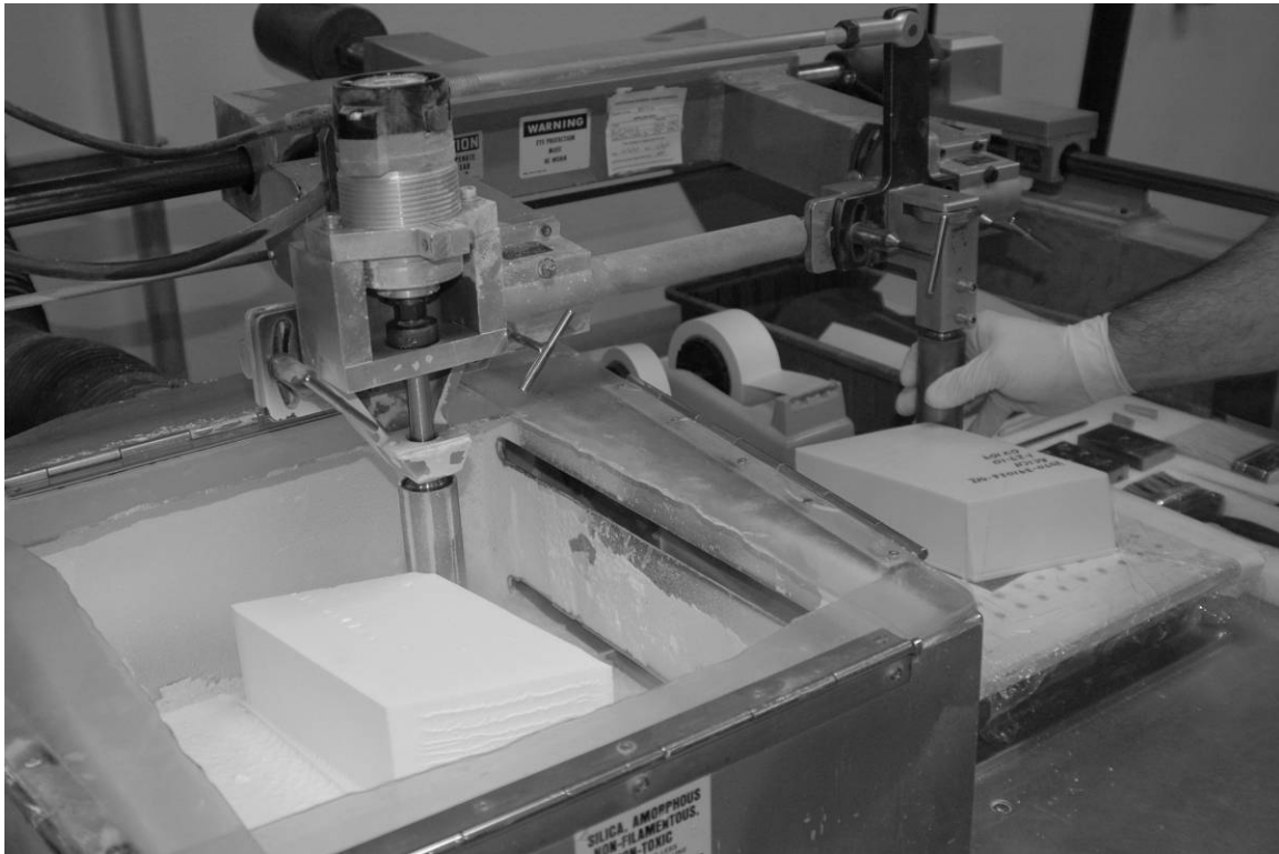
Figure A-4. Tile technician, Sean Druck, using Contour Milling Machine, March 10, 2010. Source: Penny Rogo Bailes.
