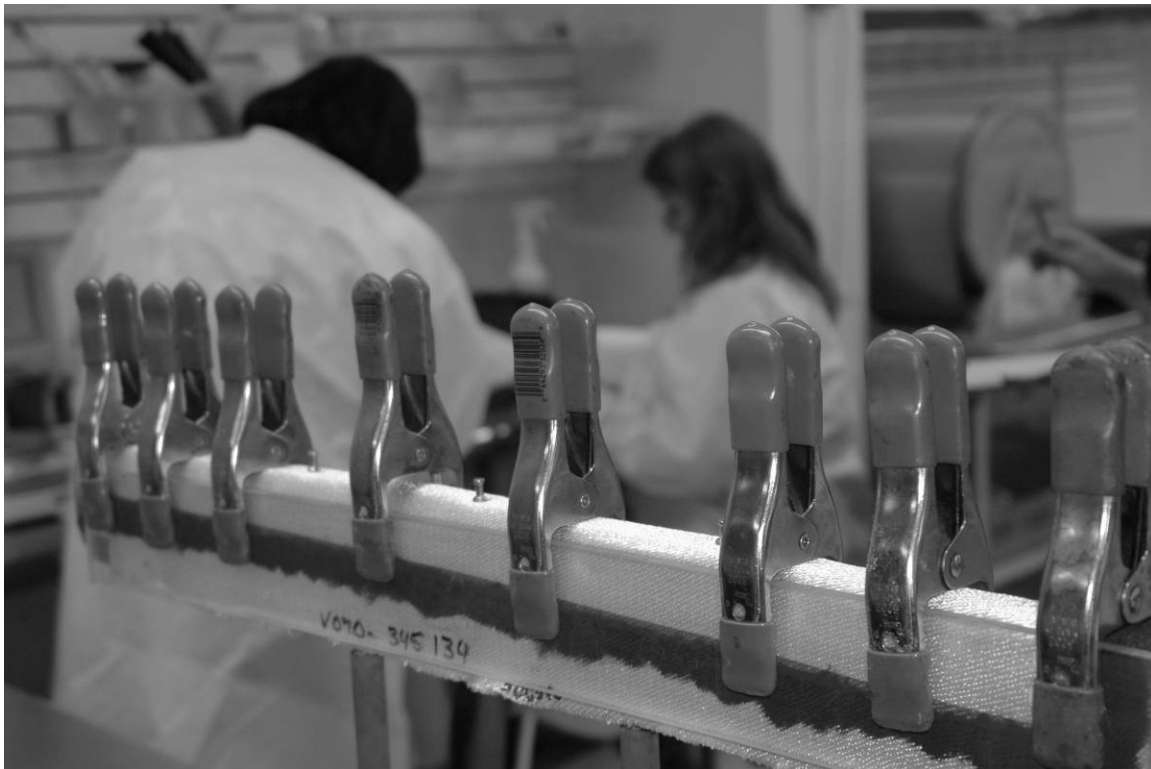
Figure A-23. Applied RTV on material for softgoods being allowed to dry, March 9, 2010. Source: Penny Rogo Bailes.
