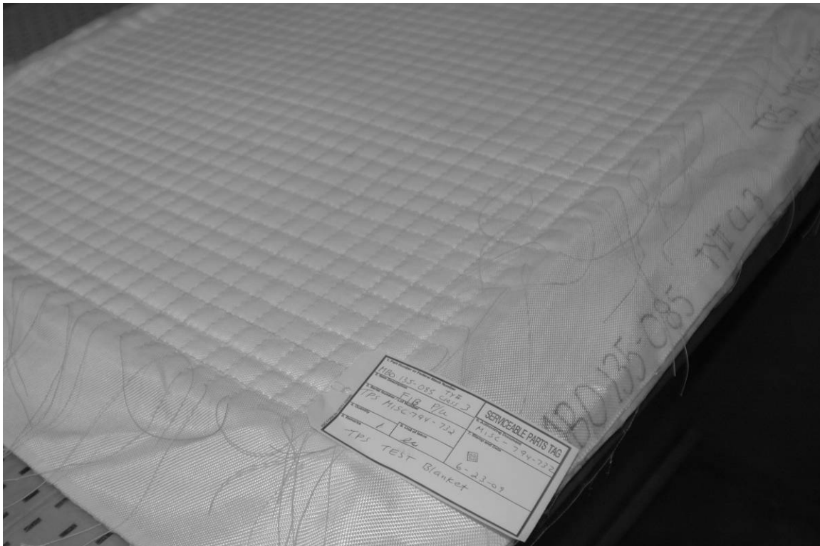
Figure A-27. FIB after sewing completed by Multi-Needle Sewing Machine, March 9, 2010. Source: Penny Rogo Bailes.
