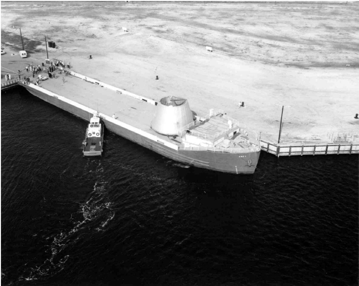
Figure D-9. A S-IV-B inner stage for a Saturn V launch vehicle on a barge docked at the Barge Terminal Facility, facing northwest, November 2, 1965.
