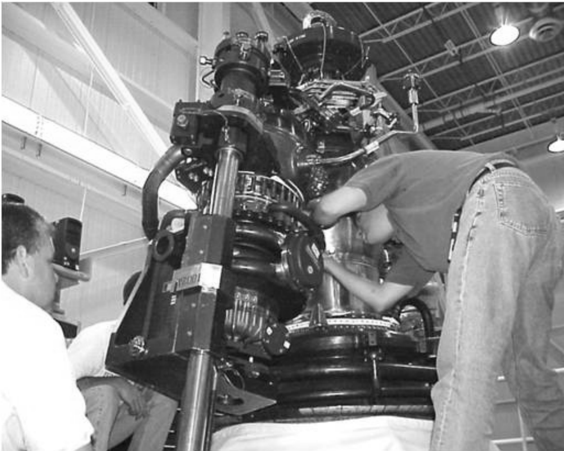
Figure A-14. A technician attaches the High Pressure Oxidizer Turbopump to the SSME, SSMEPF, looking northeast, December 2005. Source: George C. Marshall Space Flight Center.
