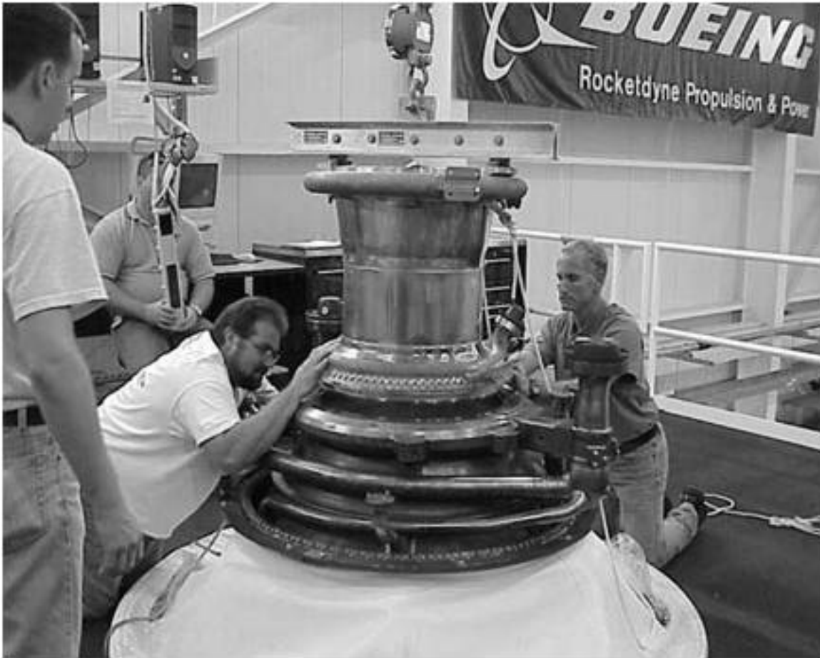
Figure A-13. Technicians attach the Main Combustion Chamber to the nozzle in the SSMEPF at Kennedy Space Center, looking northeast, November 2005. Source: George C. Marshall Space Flight Center.
